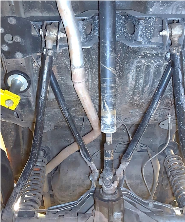
Recommended custom exhaust routing
